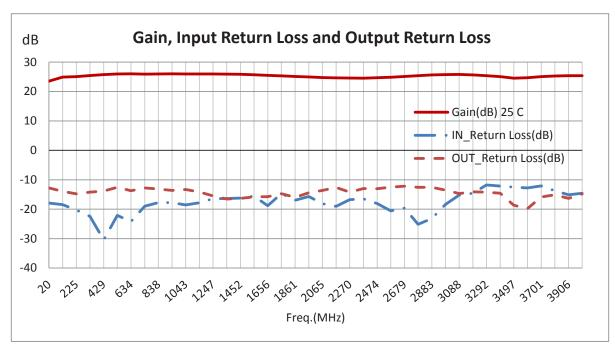
26 dB Gain Block Amplifier Operating From 50 MHz to 4 GHz with 23 dBm P1dB and SMA from Fairview Microwave is in-stock and available to ship same-day. All of our RF/microwave products are available off-the-shelf from our ISO 9001:2008 certified facilities in Lewisville, Texas. Fairview Microwave is RF on-demand.
