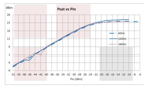
40 dB Gain Limiting Amplifier Operating From 6 GHz to 18 GHz with -20 to +15 dBm Pin, 19 dBm Psat and SMA from Fairview Microwave is in-stock and available to ship same-day. All of our RF/microwave products are available off-the-shelf from our ISO 9001:2008 certified facilities in Lewisville, Texas. Fairview Microwave is RF on-demand.
